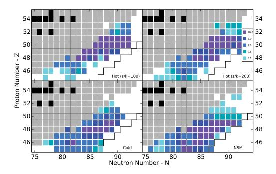
Figure 1: Maximum sensitivity measures  $F_{max}(Z, A)$  for FRDM nuclear masses (variation by  $\pm 1.0$  MeV) near the N = 82 closed shell for four *r*-process trajectories from [11]. Black squares are stable isotopes and gray shading indicates the region of measured nuclear masses from the 2012 AME. An estimated accessibility limit for FRIB is shown as a black line [19].
