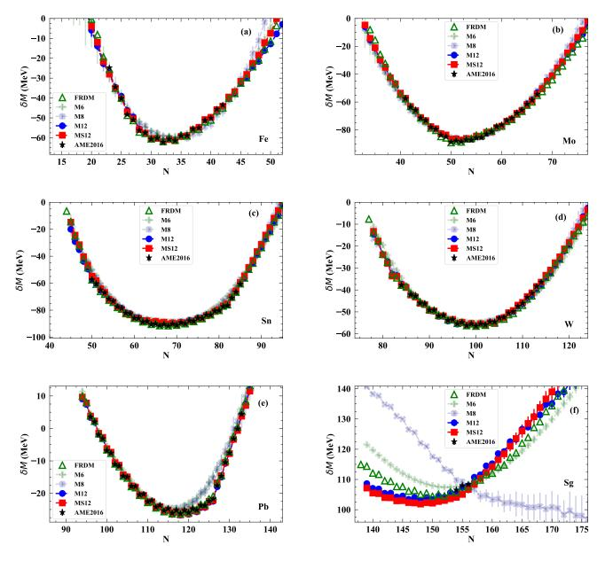
FIG. 2: Comparison of several MDN calculations—M6 (green pluses), M8 (dark blue x-es), M12 (blue circles), MS12 (red squares)—to the AME2016 (black stars) and FRDM2012 (green open triangles) for selected mass chains: (a) Fe, (b) Mo, (c) Sn, (d) W, (e) Pb, and (f) Sg.
