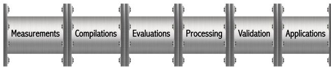
FIG. 1: Schematic showing technical components of the nuclear data pipeline toward production of libraries used by applications. Schematic example of a linear data pipeline showing how the components of the pipeline contribute to the production of data libraries used by applications. Given the multi-disciplinary nature of nuclear data, some activities may involve more than one component.
